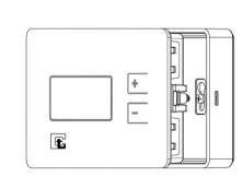
5) Attach the Campini thermostat plate to the wall.
